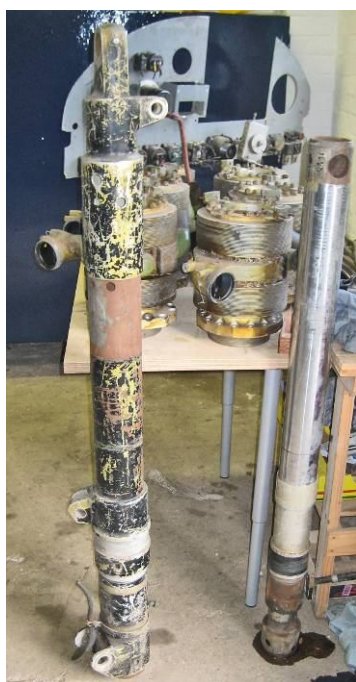
On the left is the Avro Lancaster main undercarriage oleo leg.
