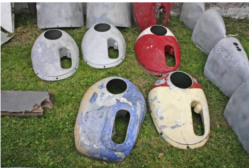
Another photo from Sunday 28 th September, all the parts were laid out on the grass for photographing before storing away in the container. Messenger and Gemini front engine cowlings, Gemini undercarriage rear cowlings.
