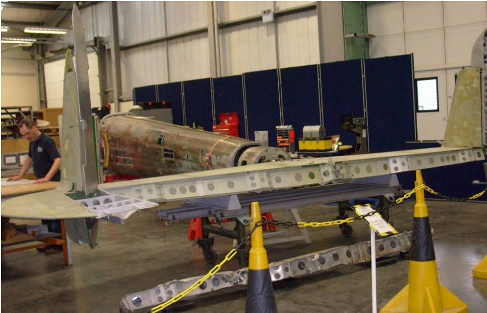
Two more from Peter's visit to Cosford, this one shows the mostly new build tail plane section for the Handley Page Hampden TB.1 P1344/PL-K
